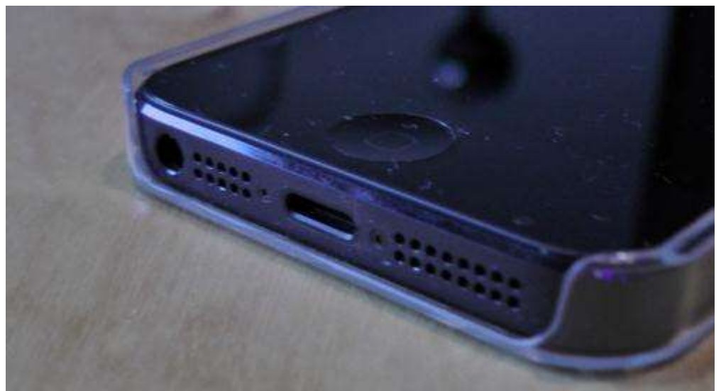
Figure 7 - Apple's new controversial "Lightning" connector
